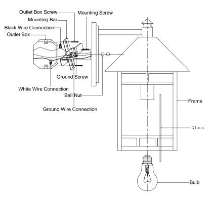
STEP 5: Use the wire connection to connect the positive and neutral wires. Connect the Ground wire to the junction box ground port.
