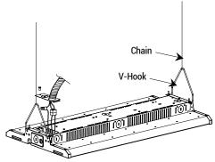
**Step3:** Take out the plate from lamp by screw driver and install the whip.
