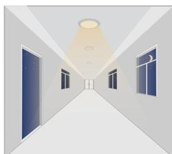
With insufficient ambient brightness, sensor turns on light and keeps it at standby dimming level even if there is no motion or presence.
