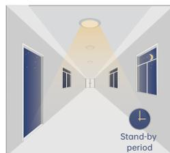
After pre-set hold time it will dim light to standby dimming level again and always keep it.
