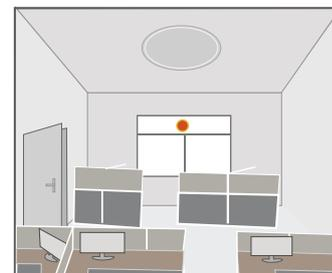
When ambient brightness is lower than preset lux level, sensor will turn on light automatically and keep dimming according to the change of the ambient brightness; when outside is getting darker, the inside will be brighter, and brighter darker.
