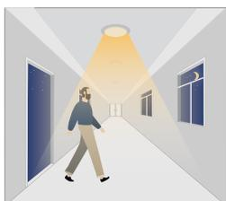
When sensor detects motion or presence it will bring the light level up to 100%.
