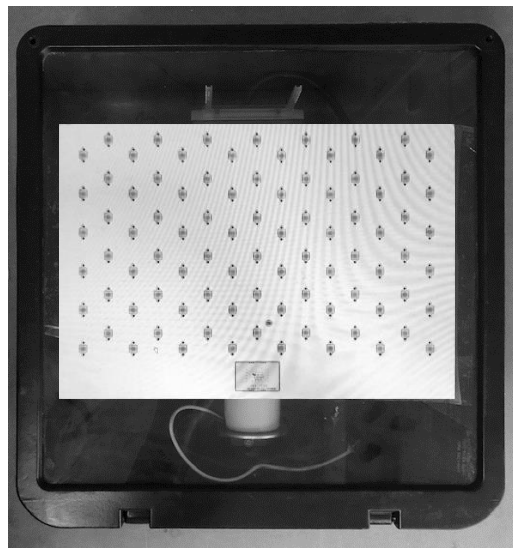
Figure 4 – Cable connected and lens closed
