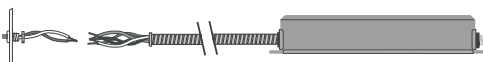
L30-C-480: Single flex conduit on each end, with test switch and plate
