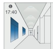
The light automatically turns on at 10% when natural light is insufficient (no motion).
