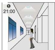
The light turns on at 100% when movement is detected.
