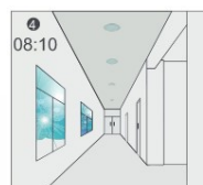
When the natural light level exceeds the set level, the light will turn OFF even if the space is occupied.
