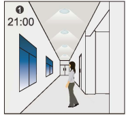
1 The light turns ON at 100% when movement is detected.
