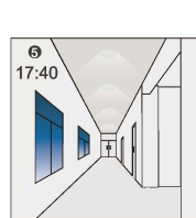
The light automatically turns on at 10% when natural light is insufficient (no motion).
