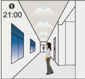
The light turns ON at 100% when movement is detected.
