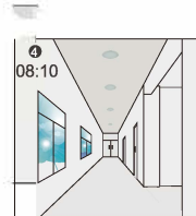
When the natural light level exceeds the set level, the light will turn OFF even if the space is occupied.
