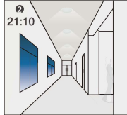
The light dims to stand-by level after the hold-time elapses.
