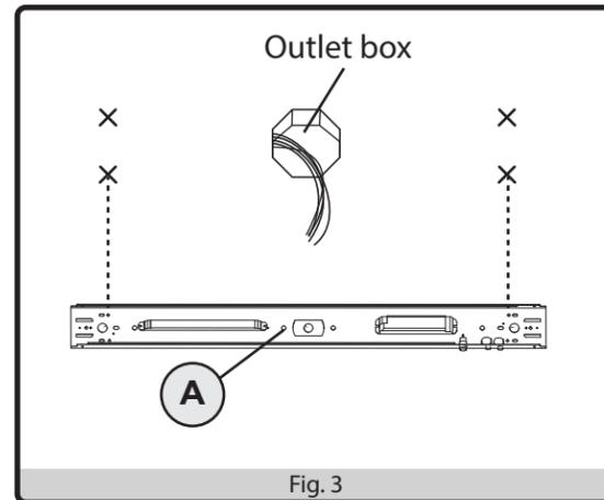
4. **DRYWALL MOUNTING:** If the mounting holes go through drywall without a stud, drill four small pilot holes using a 1/8-in. drill bit (not included), and install drywall anchors (CC) into the holes with a hammer (not included).
