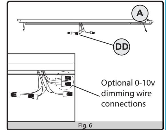
7. Re-connect the wire connectors between the fixture plate (A) and lens (B)
