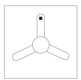
Stick the adhesive-backed balancing weight on the top center of the blade directly in line with the balancing clip.Add more weight if needed to get a smooth-running fan.
