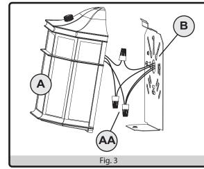
4. Insert the upper tab on mounting plate (B) through the slot on the back of the fixture (A) housing, then swing the bottom towards the mounting surface until flush. Replace the thumbscrew from step 1 above by turning clockwise back into the fixture until fixture is fully secured.
