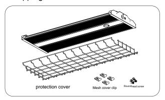
2.Insert the provided chips(4 pcs) onto the wire guard.
