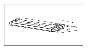
4. Put the desired diffuser into the chanel.
