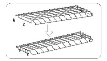
3. Fasten the chips by screws into the prepunched holes of fixture body.
