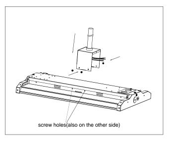
4. Install the two side-covers of the bracket with screws to hide the wires.
