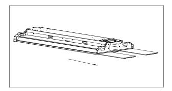
5. Reattach the end-cover to the fixture body and fix it with screw.
