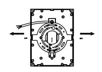
Step 3: Screw the bracket onto the wall.
