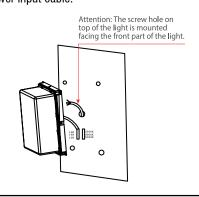
**Step 3:** Screw and fasten the light to the wall with 4 KA5X12 screws on the 4 corners of the light.
