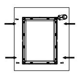
Step 4: Screw and fasten the outer frame back to the light with one screw on the top and two screws at the bottom.
