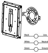
**Step 5:** Screw and fasten the light to the bracket by aligning the holes, and screw on both sides.
