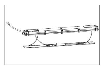
8. Reattach LED tray to fixture by reversing step 5.
