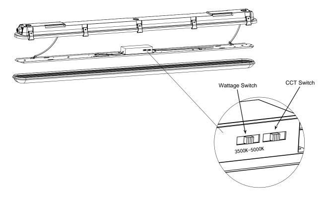
The end users may adjust the color temperature and lumen output respectively by the two DIP switches buttons integrated into the driver. Each DIP switch is accommodated with 3 options (left, middle and right), corresponding to 3 color temperatures and 3 wattages respectively, which can perform the desired color temperature and lumen output combination.
