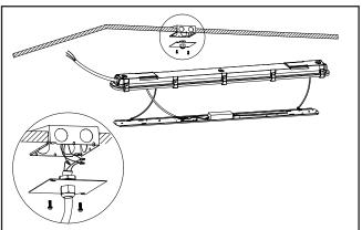
7. Reattach LED tray to fixture by reversing step 4.
