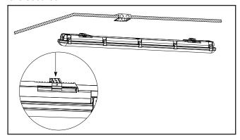
4. Without touching LED boards, detach LED tray from fixture. The tray will be suspended by safety cables.
