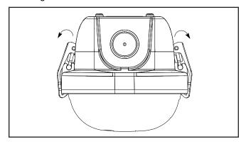
Secure mounting clips to housing recesses by firmly pressing them into place until both sides of the clip are secured.
