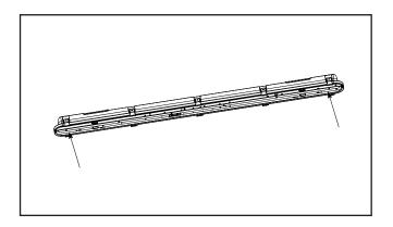
8. Secure lens to housing with lens latches.
