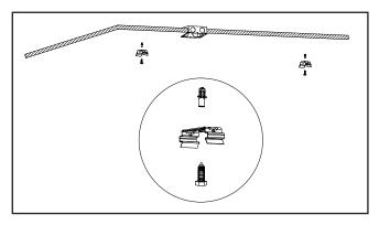
3.Release latches by pulling top of latch away from housing. Set the lens aside.
