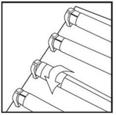
Twist T8 lamp to secure until resistance is met. Make sure light emitting side is facing out. Replace all lamps. Black lines on lamp to match up with slots of the socket. Installation Instructions
