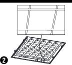
2. Feed the main AC wire in driver terminal block respectively, connect the panel light and driver.
