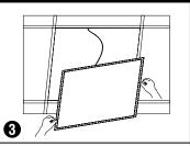
3. Fix the panel light into plaster ceiling.
