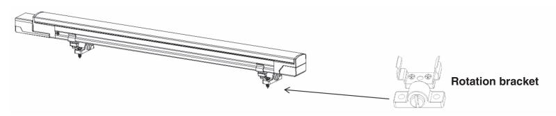
2.) Attach the bracket to a magnetic surface so that no screws are necessary. Insert the LiteBar into the clip.
