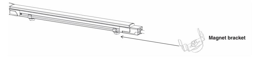
3.) Insert the LiteBar into the clip. Fix the bracket to the mounting surface with 2 screws.
