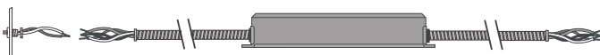
L25-DC-CEC: Dual flex conduit on each end, with test switch and plate
