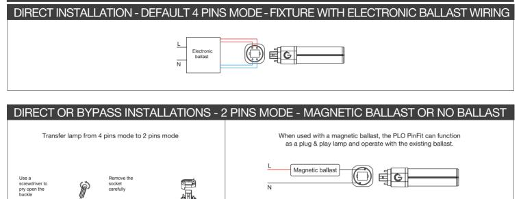
If the ballast is not compatible, it can be bypassed and the lamp can run directly off line voltage.
