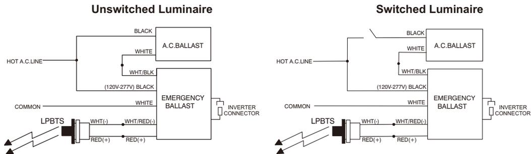
**EMERGENCY BALLAST INSTALLATION LOCATION:** FireHorse emergency ballast can be mounted in the ballast channel compartment, on top of the luminaire or remotely.
