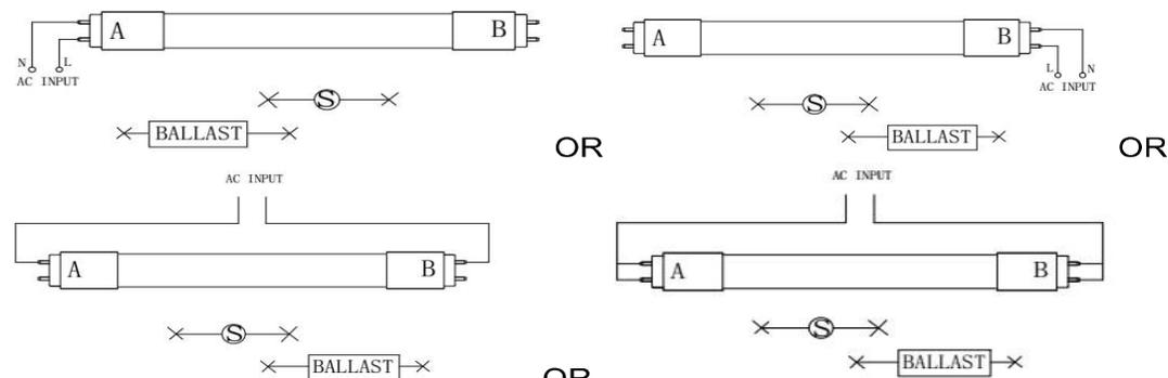
Voltage Input: AC120-277V 50/60Hz
