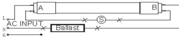
If no starter is present, simply disconnect the wires before and after the ballast.
