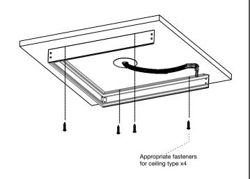
3.Put the wire conduit hose as close as possible to the surface mount opening before placing/inserting the luminaire into it partially.Make all electrical connections according to local code and make s ure wire conduit hose is long enough for wiring connection job.
