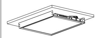
5. Place the last frame into the slots ,then slightly slide the last frame to the left , make sure it get locked tightly, join the last frame to the rested frames by fastening them together with appropriate fasteners .
