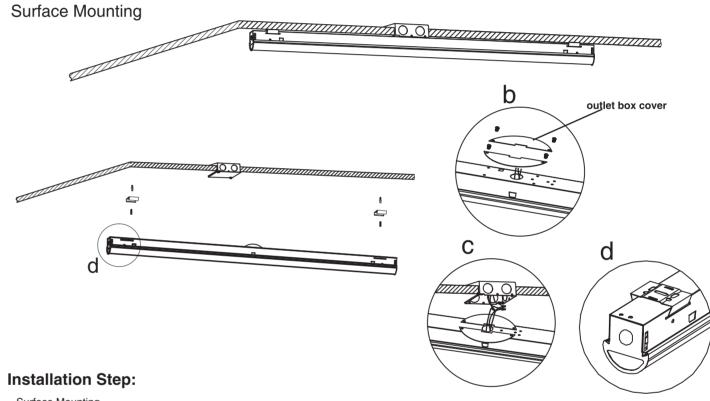
Step1: Secure the provided brackets onto the ceiling with the provided accessories and screws.
