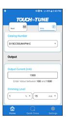
**Universal**<sup>™</sup> Lighting Technologies 5. Scroll down to adjust Dimming Curve, Full Bright Control Voltage, Minimum Dim Control Voltage, and Dim-To-Off-Control Voltage if needed. \* *This step is not required.*
