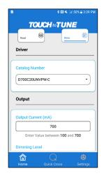
Step 3: Position the Android device over the RFID tag located on the EVERLINE driver. Listen and watch for confirmation that the driver is tuned.
