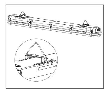
4.Release latches by pulling top of latch away from housing. Set the lens aside.
