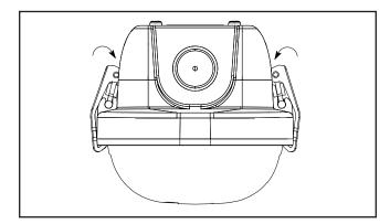
6.Assemble the PG13.5 waterproof cable connector and position it in the appropriate end of the fixture housing. Bring an (owner-supplied) 6-10 millimeter diameter electrical cable through the PG13.5 waterproof cable connection. Include 0-10V dimming conductors in the cable if 0-10V dimming is desired. Make appropriate electrical connections with the driver.
