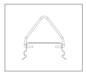
3.Hang fixture from customer supplied chain using V-brackets.
