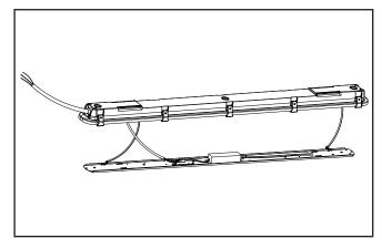
Include 0-10V dimming conductors in the cable if 0-10V dimming is desired. Make appropriate electrical connections with the driver.
