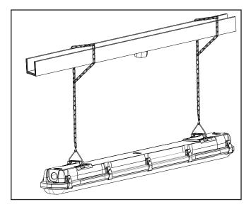
2.Secure mounting clips to housing recesses by firmly pressing them into place until both sides of the clip are secured.
