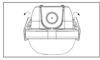
2.Secure mounting clips to housing recesses by firmly pressing them into place until both sides of the clip are secured.
