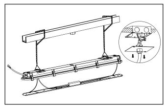
9.Secure lens to housing with lens latches.
