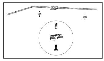
3.Release latches by pulling top of latch away from housing. Set the lens aside.
