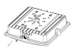
3. If you need to use the surface-mounted installation, a circle of glue is needed around the edge of the fixed plate.
