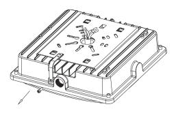
PS: Wire the dimming wires (DIM+/DIM-) if needed, otherwise hide them in junction box.
