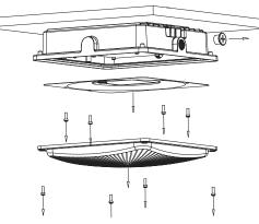
7. Put back the reflector and lens, make sure no wires are pinched or exposed during the whole process.
