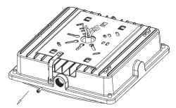
3. Buckle the connecting plate into the clips, and seal 3/4" screw knockout on the top with glue. 4. Slide fixture back into the connecting plate
