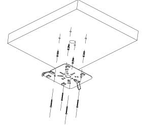
Buckle the connecting plate into the clips and connect the wires as shown below.
