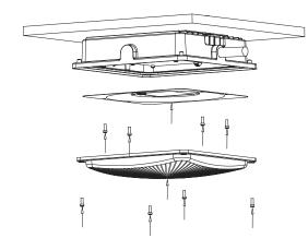
2. Fix the connecting plate onto the ceiling.
