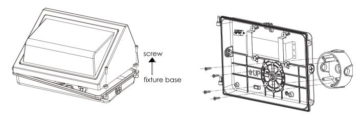
Method 2: Drill holes at the required three mounting points, mount the fixture by securing mounting screws (not provided) through the drilled holes, and seal the screw heads with appropriate waterproofing material.
