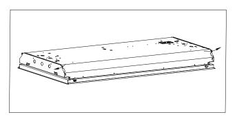
3. Lay fixture into T-grid.
