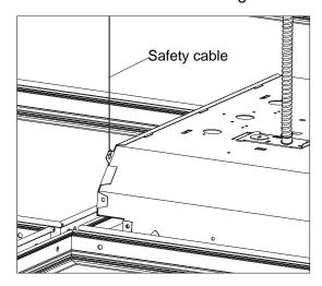
5. Ensure that the wiring of the last fixture in the row is properly terminated. Then make all electrical connections to the fixture. Attach the wiring access cover plate.
