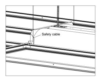
5. Ensure that the wiring of the last fixture in the row is properly terminated. Then make all electrical connections to the fixture. Attach the wiring access cover plate.
