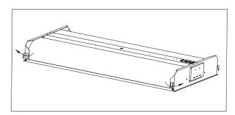
3. Lay fixture into T-grid.
