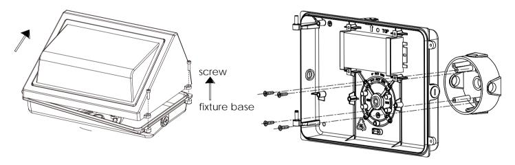
Method 2: Drill holes at the required three mounting points, mount the fixture by securing mounting screws (not provided) through the drilled holes, and seal the screw heads with appropriate waterproofing material.
