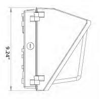
Dimensions Length: 14.25 in. Width: 9.24 in. Height: 7.55 in. Weight: 8.04 lbs
