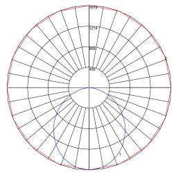
$\label{eq:maximum Candela} \begin{tabular}{ll} Maximum Candela = $1671.01$ Located At Horizontal Angle = $10$, Vertical Angle = $5$ $\# 1$ - Vertical Plane Through Horizontal Angles (0 - $190) [Through Max. Cd.] $$\# 2$ - Horizontal Cone Through Vertical Angle (5) [Through Max. Cd.] $$$
