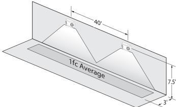
Using multiple LED-52 (4W) units mounted at a typical 7.5' height delivers 30' on center spacing with a 6' wide path of egress.
