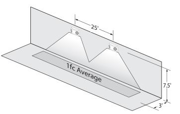
Using multiple LED-51 (2W) units mounted at a typical 7.5' height delivers 23' on center spacing with a 6' wide path of egress.
