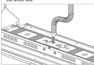
6.Insert the wire terminal joint to the wire entry.Installation completed.
