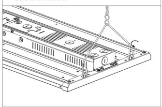
3. Hook up the chain on the ceiling anchor.
