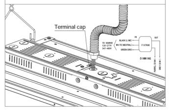
5.Insert the terminal cap and wires into the driver box.
