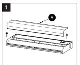
Remove channel cover (C) from channel (B) by squeezing the cover till it releases from channel boby tabs. Remove the parts bag.
