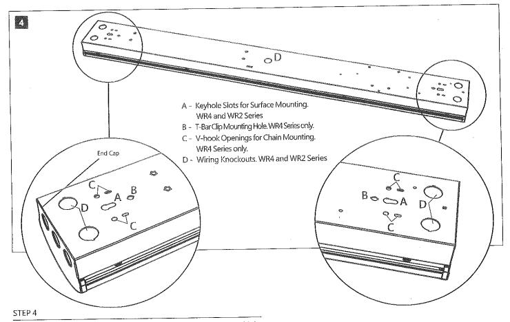
For single luminaire installation proceed to the next Step. For multiple luminaire installation, insert customer-supplied chase nipple and lock nuts into the knockout on the end cap located on each end of the luminaire. See Figure 6.
