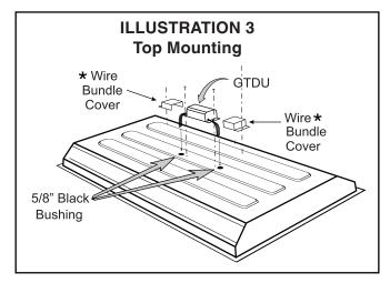
\* For installation on top of the fixture, wire bundle covers (RMC-60) may be required by state or local codes. These covers are available from the manufacturer as an accessory kit and must be ordered separately. Call your local distributor or the factory for complete information.
