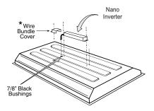
If the application requires the ELI-S-10 to be mounted on top of the luminare please use Model ELI-S-10C instead or wire bundle cover kit (RMC-60). Please note, the RMC-60 kit contains enough parts to install two products.
