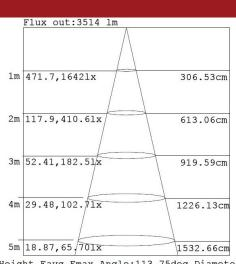
Height Eavg, Emax Angle:113.75deg Diameter Note: The Curves indicate the illuminated area and the average illumination when the luminaire is at different distance.
