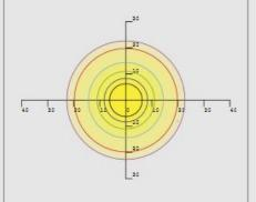
Mounting Height 10m, 0 Tilt, 20LUX-0.2LUX
