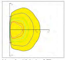
Mounting Hight 4m, 0 Tilt, 50LUX-5LUX
