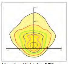
Mounting Hight 4m, 0 Tilt, 50LUX-5LUX
