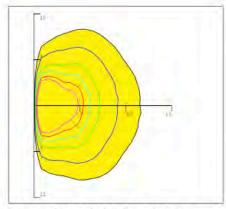
Mounting Hight 4m, 0 Tilt, 50LUX-5LUX
