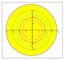
Mounting Height 20m, 0 Tilt, 50LUX-5LUX
