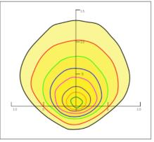
Mounting Hight 4m, 0 Tilt, 50LUX-5LUX
