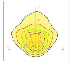
Mounting Hight 4m, 0 Tilt, 50LUX-5LUX
