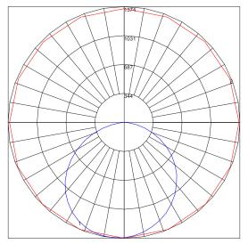
Maximum Candela = 1374 Located At Horizontal Angle = 270, Vertical Angle = 5 # 1 - Vertical Plane Through Horizontal Angles (270 - 90) [Through Max. Cd.] # 2 - Horizontal Cone Through Vertical Angle (5) [Through Max. Cd.]
