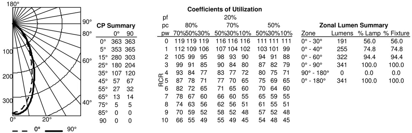
LTKMSBK 90CRI MW, 2700 K LEDs, input watts: 5, delivered lumens: 389, LM/W = 77.8, test no. ISF 36854, tested in accordance with IESNA LM 79-08
