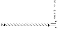
2. Install the 4 plastic anchors 46 1/2" apart and 3.189" apart, then screw into each anchor. Spacing between ceiling and cap nut should be at least 1/3".
